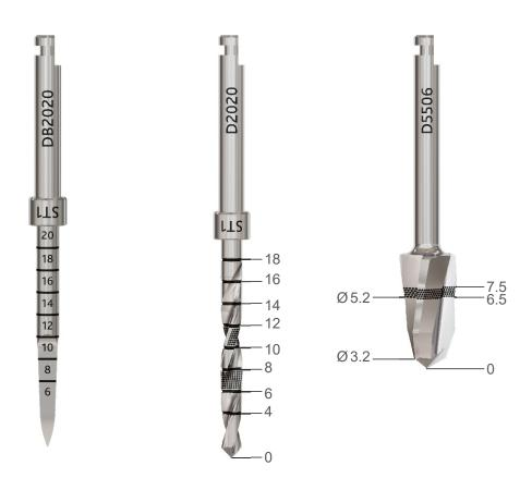
Tapered drills have V-shaped tips, for better correlation with the implant, 3 cutting edges offer good stability. The tapered shape reduces frictional heating. Variable helix for enhanced drilling control and twisted flute for bone extraction. Angled back cutting edge allows compressing of bone when drilling in counter-clock wise (reverse).
