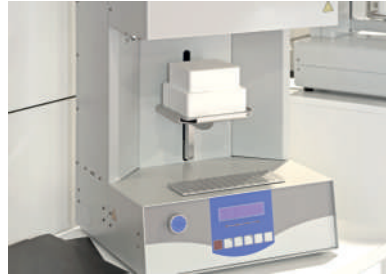
Sinter the finished prosthesis according to the recommendations of the raw material producer. Post-process as normal and dye, if required.
