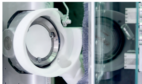
Option b. Choose raw material for prosthesis and place to milling machine.
