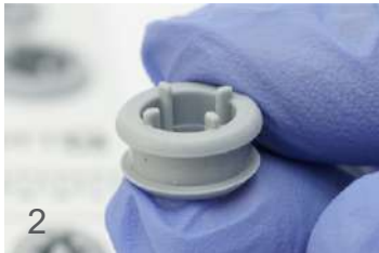
1, 2 photo. Top part of the grommets is raised or has "spikes".
