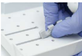
Place the grommet directly into the corresponding holes, ensuring a distinct 'click' is both heard and felt. Insert both grommets from the same side for proper alignment.
