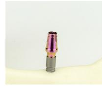
Insert implant via CRE with insertion tool for external platform. Use insertion tool ITES/ITE/ITEL/ITEXL for ratchet TW50 with torque up to 40 Ncm
